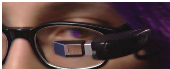
Figure 1: The MicroOptical head-up display mounted on eyeglasses.
