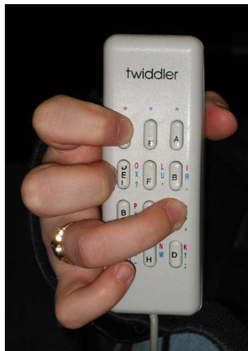
Figure 2: The Twiddler one-handed chording keyboard.
